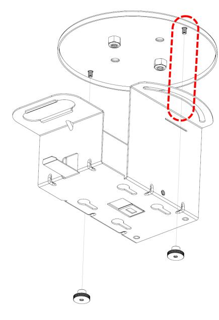
NOTE: Align the threaded studs with the curved slots in the bracket.
