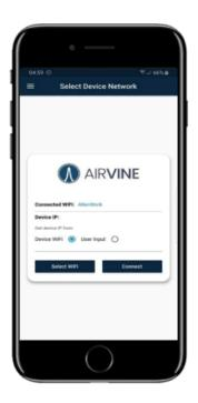
Connect the WaveTunnel node to be configured via the default management SSID which is "avb\_[Device MAC]".
