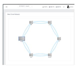
To manage the WaveTunnel device, you can select any device on the network from the drop-down list in the WEB GUI or Mobile App.
