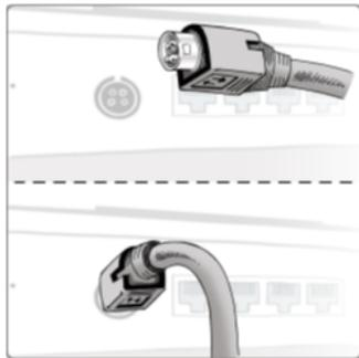
For model **2041DC**, the flat side of the power connector is up.
